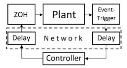
Fig. 1. A system with network-induced delays
